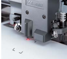
The Optical sensor comes with a LED pointer (Light pointer) for ease of use.
