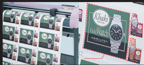
Cutting with the CG-FX series as a Print-cut solution
