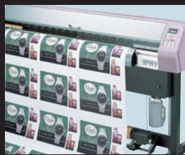
Nesting with the Inkjet plotter JV3 series
